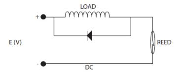
When the circuit is alternating, the diode cannot be used. Therefore an arc suppression unit must be used; in general this is a block of resistances and capacitances connected together in series and in parallel with the reed.
