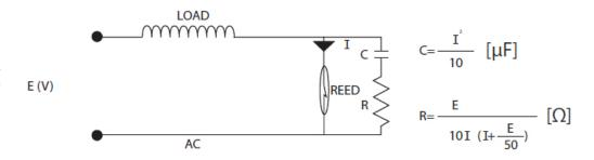
When the contact remains open for a long time, it is advisable to install a varistor in parallel with the load.
