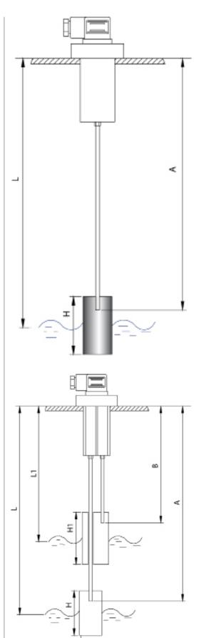
L-LI = 100 mm A-B = 90 mm H = 35 (L = 90 mm) H = 45 (L = 100 mm) H = 55 (L = 110 mm) H = 60 (L = 120 - 500 mm) H = 90 (L = 501 - 1000 mm) HI = 35 (LI = 90) HI = 45 (LI = 100) HI = 70 (LI = 120 - 1000 mm)
