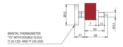
Maximum pressure: see page 33 Maximum tightening torque: 10 Nm
